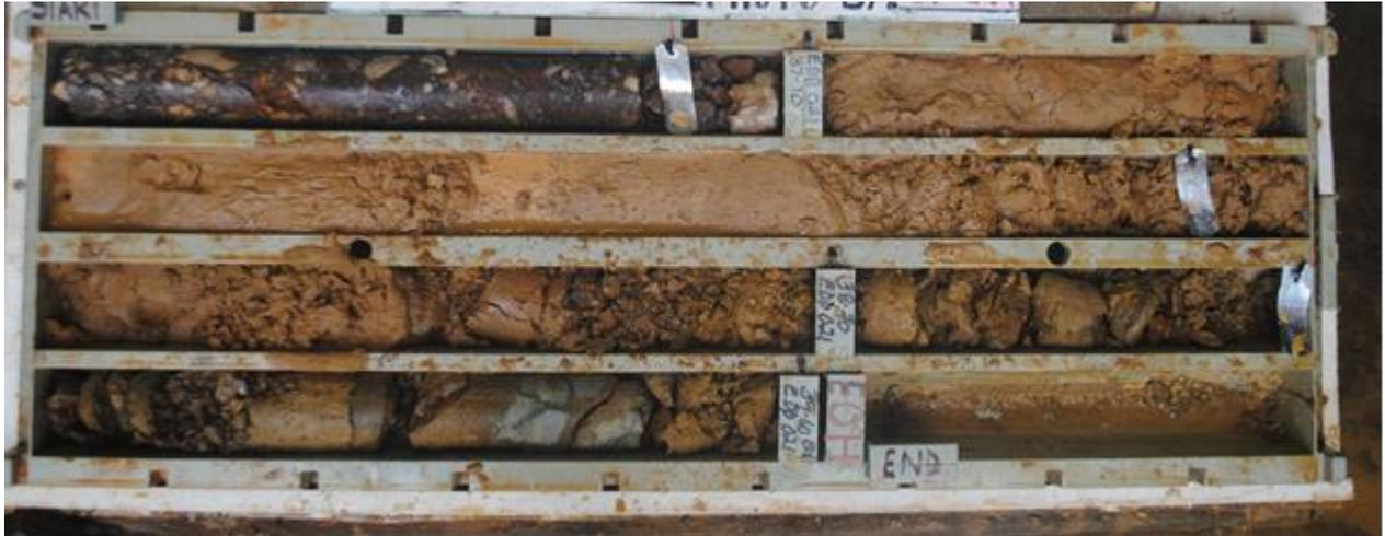
All 6 holes were drilled, as expected, in highly oxidised rock with a stock-work of numerous narrow veinlets of mineralised quartz, iron oxide and manganese oxide.
